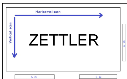
Fig. 1 Normal scan (Pin24, Reverse = Low or NC)
