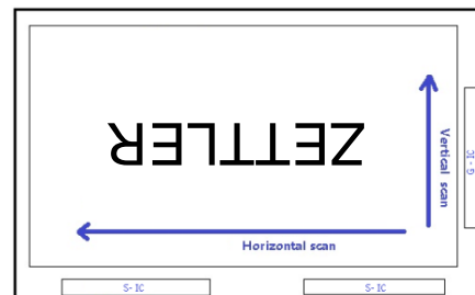
Fig. 2 Reverse scan (Pin24, Reverse = High)
